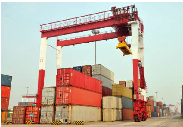
Figure 61 Gantry crane for moving shipping containers
