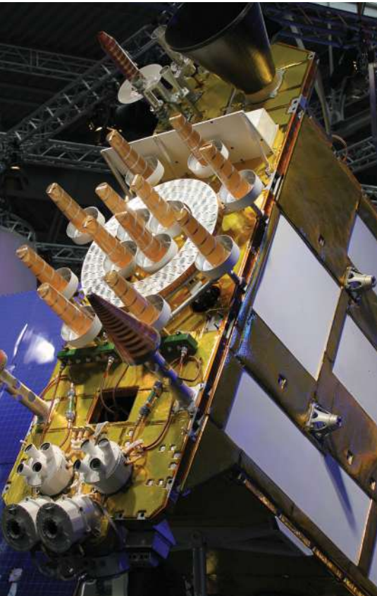
Figure 31 GLONASS-M satellite in final manufacturing
